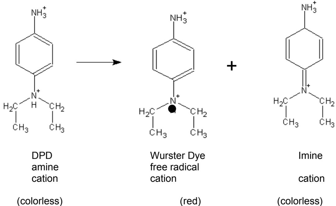
DPD is a 2+ cation, usually used as a sulfate salt. Rapid reaction with Chlorine produces "Wurster Dye", a red 2+ cation which is also a free radical. This dye further oxidizes to a colorless Imine product. With small amounts of chlorine near neutral pH, Wurster dye is the dominant product. At higher levels, the unstable, colorless Imine is produced and rapid fading of the colored solution occurs.
